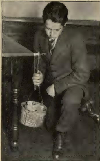
FIG. 33. With this arrangement the pail travels more slowly than the hand. Will it seem heavier or lighter than with the arrangement shown in Figure 32?
